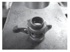
2. Place the rocker arm beneath the press, and put the new bearing or bushing squarely on the fulcrum bore. The part number of the bearing MUST be facing outward. For bushings, there is no particular orientation. Be certain the bearing or bushing is as flat and level as possible.
